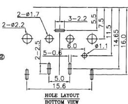
Unless specified, the tolerance is  $\pm 0.2$ mm
